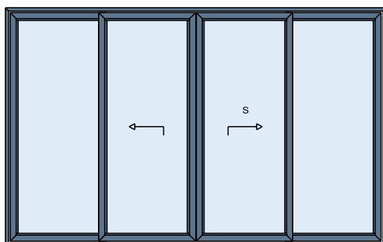
SCU SCI50TH Standard Two Rail Four Leaf Lift and Slide Door
